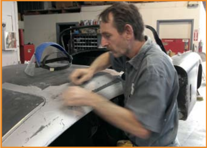
Above our hands-on body shop manager, Mel, works over a rear cowl after metallic filler has been applied.
