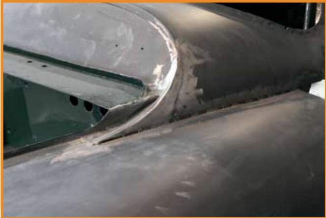
Above our hands-on body shop manager, Mel, works over a rear cowl after metallic filler has been applied.
